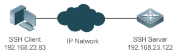
Figure 9-5 Networking Topology of SSH File Transfer
