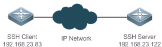
Figure 9-6 Networking Topology of SSH Client Application
