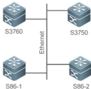
Figure 6-18 IS-IS GR Topology
