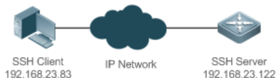
Figure 15-4 Network Topology for Public Key Authentication of SSH Users
