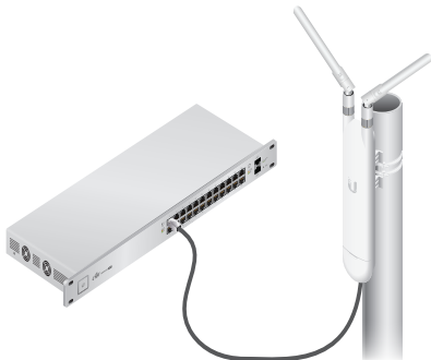
Connected to UniFi Switch, model US-24-250W
