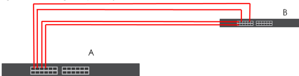
Figure 152 Trunking Example – Physical Connections
