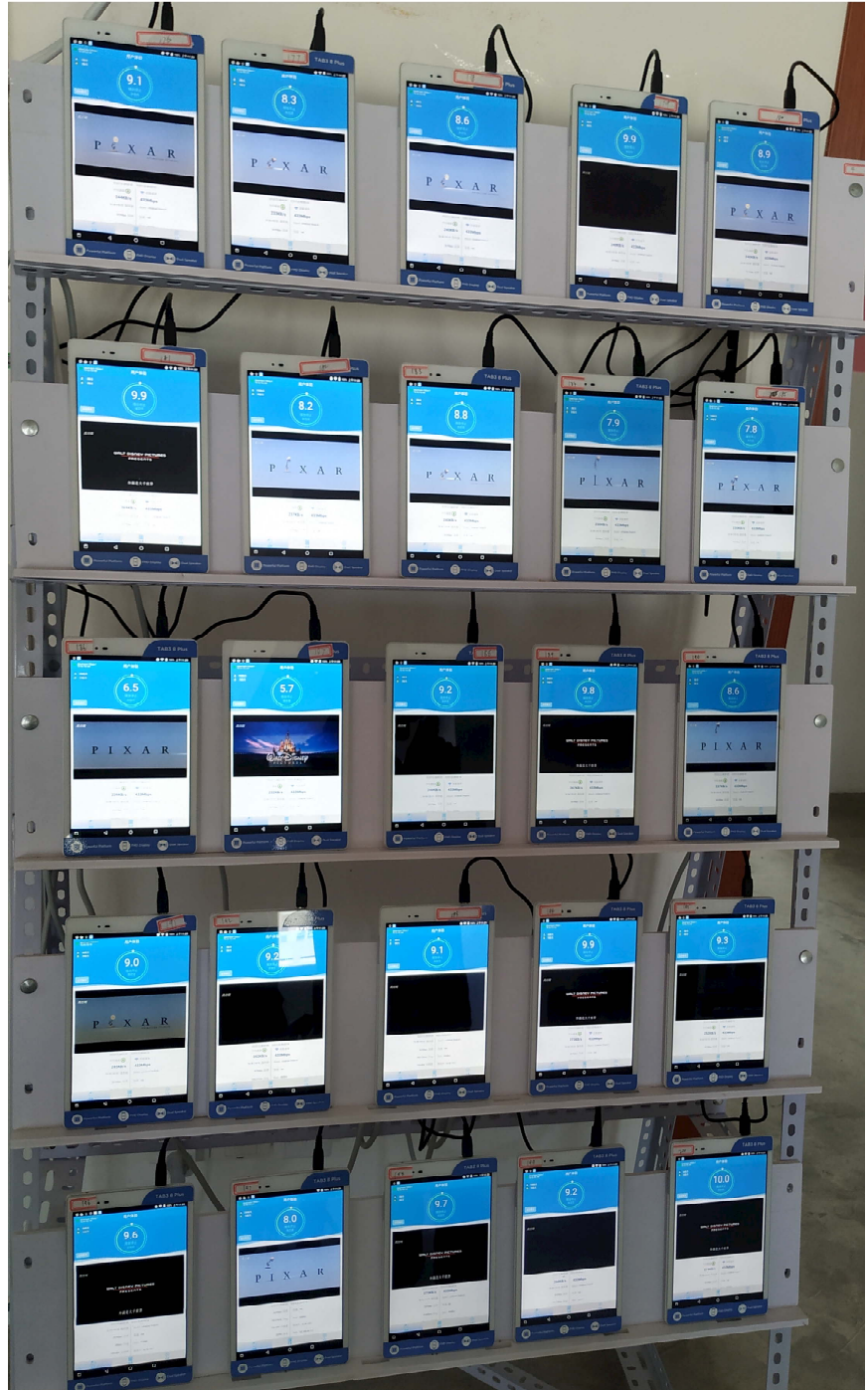
Note: The test includes four of this rack in different directions to the AP. Each rack had 25 1x1:1 Android tablets.
