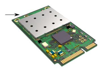
Attach antenna cable to the connector on the module:
