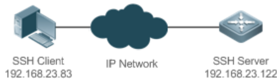
Figure 15-5 Networking Topology of SSH File Transfer
