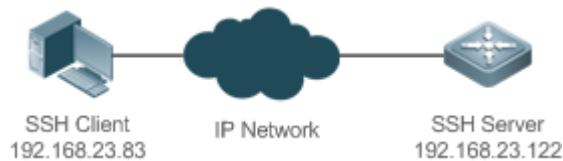
Figure 15-5 Networking Topology of SSH File Transfer
