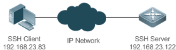
Figure 15-1 Networking Topology of SSH Device Management
