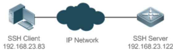
Figure 15-1 Networking Topology of SSH Device Management
