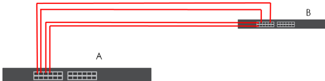
Figure 156 Trunking Example – Physical Connections
