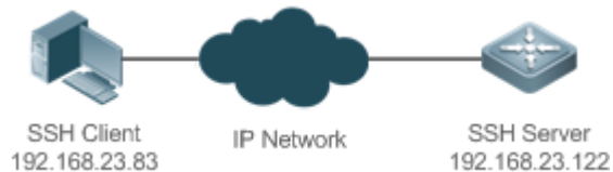
Figure 10-5 Networking Topology of SSH File Transfer
