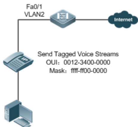
Figure 8-1 Networking When the Voice VLAN Works in Automatic Mode
