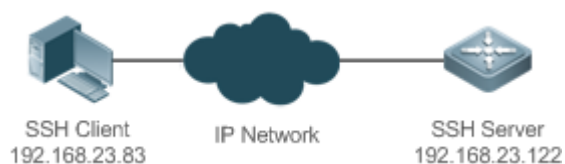
Figure 10-1 Networking Topology of SSH Device Management
