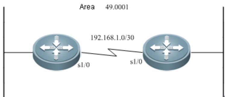
Figure 7 IS-IS point-to-point serial link configuration
