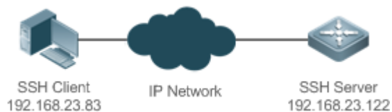
Figure 14-4 Network Topology for Public Key Authentication of SSH Users
