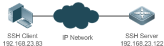
Figure 11-1 Networking Topology of SSH Device Management
