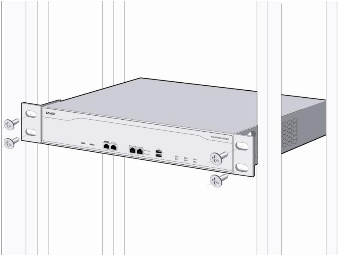
Figure 3-3 Step 2-Mounting the Router on a Rack
