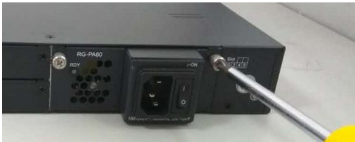
Figure 3-9 Tightening the Fastening Screws
