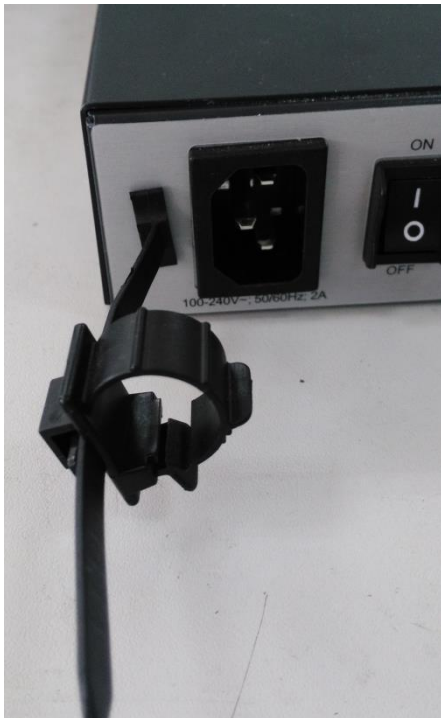
Figure 3-4 Inserting the Buckle into the Mounting Hole
