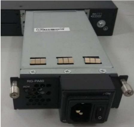
Figure 3-8 Flushing the Module and the Router Base
