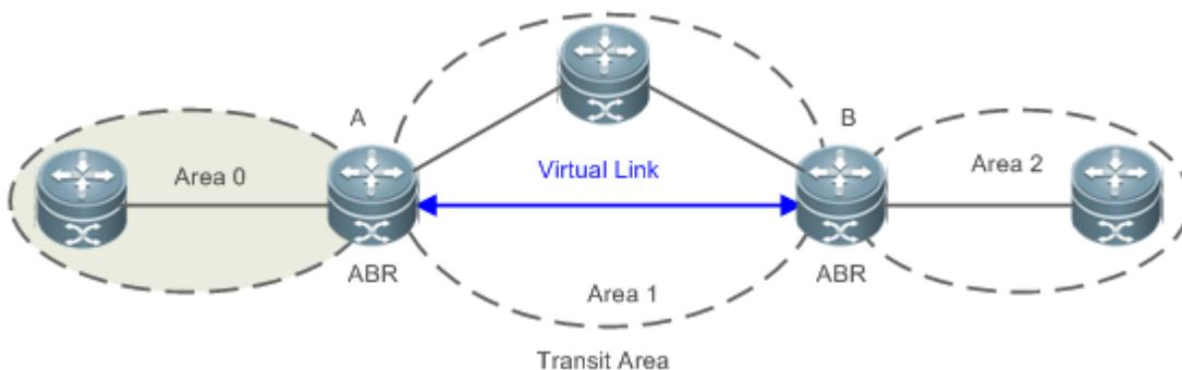
As shown in Figure 2-3, a virtual link is set up between A and B to extend area 0 to B so that area 0 can be directly connected to area 2 on B. Area 1 is a transit area, A is an ABR of area 1, and B is an ABR of area 0 and area 2.
