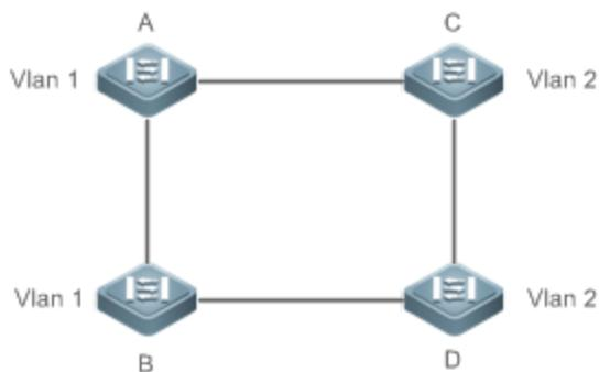
If the link from Device A to Device B through Devices C and D costs less than the link from Device A direct to Device B, the link between Device A and Device B enters the discarding state (as shown in Figure 9-13). Since Devices C and D do not include VLAN 1 and cannot forward data packets of VLAN 1, VLAN 1 of Device A fails to communicate with VLAN 1 of Device B.
