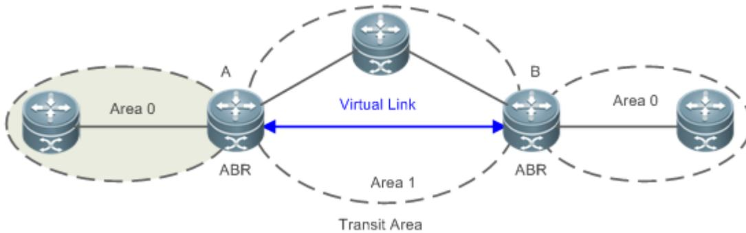
As shown in Figure 3-3, a virtual link is set up between A and B to connect two separated parts of Area 0. Area 1 is a transit area, and A and B are ABRs of Area 1.
