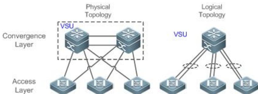
In the above VSU network structure, the member devices form a logical entity through internal links and the access layer devices are connected to the VSU through aggregated links. In this way, there is no layer 2 loop between the access and convergence layers.
