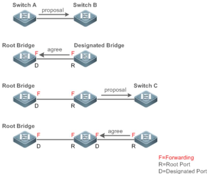
**i** The above handshake process is implemented only when the connection between ports is in point-to-point mode. To give the devices their full play, it is recommended not to enable point-to-point connection between devices.
