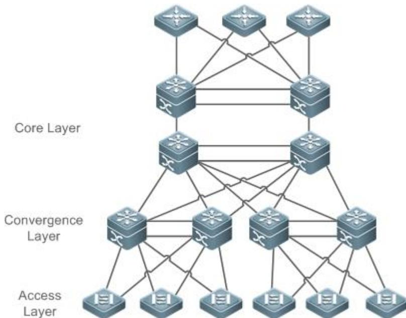
Virtual Switching Unit (VSU) is a kind of network system virtualization technology that supports combining multiple devices into a single virtualized device. As shown in Figure 7-2, access, convergence and core layer devices can respectively form VSUs, and then these VSUs connect to one another to form an end-to-end VSU network. Compared with traditional network, this networking can:
