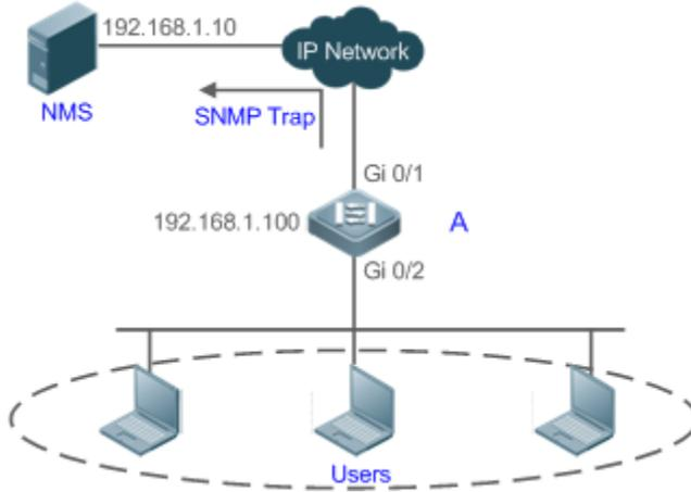
The figure shows an intranet of an enterprise. Users are connected to A via port Gi0/2.
