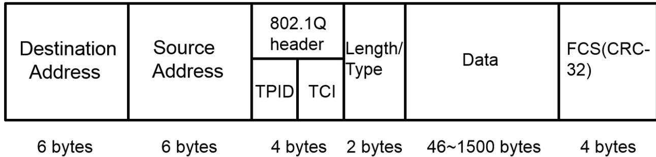
As shown in Figure 2-3, the 4-byte 802.1Q header contains 2-byte Tag Protocol Identifier (TPID) whose value is 0x8100 and 2-byte Tag Control Information (TCI). The first three bits of the TCI indicate the 802.1P priority.
