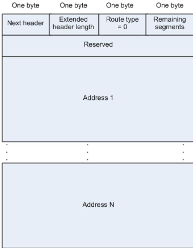
The following example describes the application of the Type 0 routing header, as shown in Figure 3-13.
