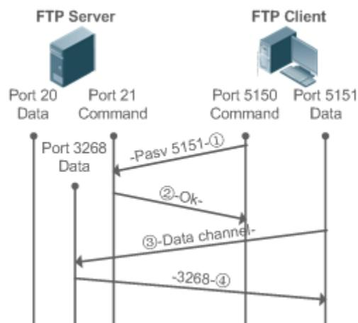
This mode is often set by the **passive** command. When a data connection is established, the FTP server is connected to the FTP client passively. This mode comprises four steps:
