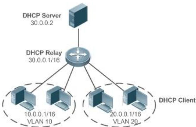
VLAN 10 and VLAN 20 correspond to the segments 10.0.0.1/16 and 20.0.0.1/16 respectively. A DHCP server with IP address 30.0.0.2 is in segment 30.0.0.1/16. To achieve management of dynamic IP addresses in VLAN 10 and VLAN 20 by the DHCP server, you only need to enable DHCP Relay on a gateway and configure IP address 30.0.0.2 for the DHCP server.
