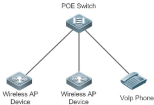
With constantly increasing functions, terminals consume more and more power. The power consumption of certain terminals exceeds the maximum power 30 W that can be provided by POE+. Consequently, these terminals have to return to the traditional power supply mode.
