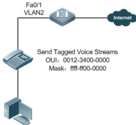
The Fa 0/1 port is connected to an IP phone that automatically obtains the IP address. After obtaining the IP address in the voice VLAN, the IP phone can be used normally. The Fa 0/1 port is required to forward both voice and data streams and isolate voice streams from data streams. The port can be configured as a trunk port. The native VLAN forwards data streams, whereas the voice VLAN forwards voice streams.
