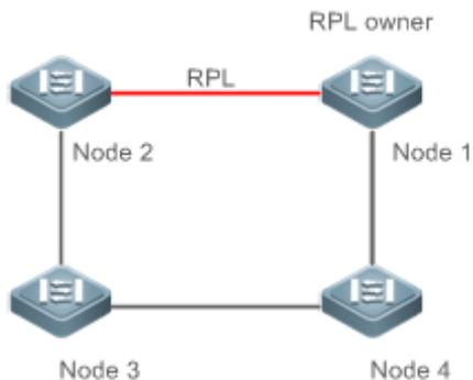
**Remarks** The four devices in the ring network are aggregation switches.
