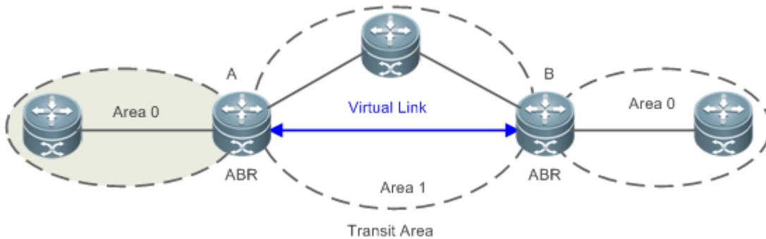
As shown in Figure 2-3, a virtual link is set up between A and B to connect two separated area 0s. Area 1 is a transit area, and A and B are ABRs of area 1.
