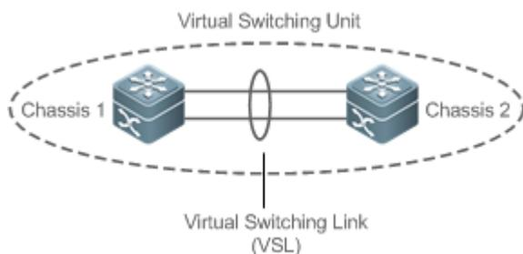
The VSL exists in the form of AP groups. The data streams transmitted through the VSL balance load among the aggregation port members according to the traffic balancing algorithm.
