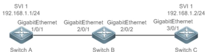
As shown in Figure 1-1, Switch A, Switch B, and Switch C form a simple L2 data switching network.
