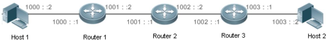
Host 1 sends Host 2 a packet specifying the intermediate nodes Router 2 and Router 3. The following table lists the changes of fields related to the IPv6 header and routing header during the forwarding process.
