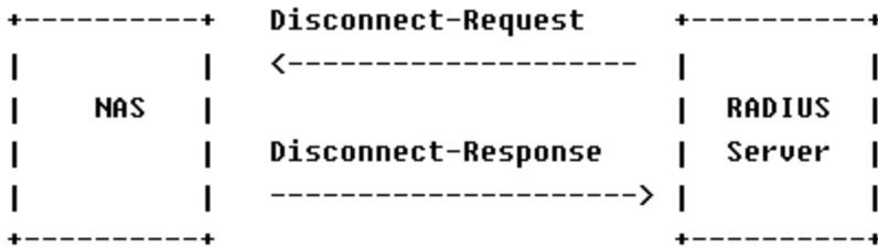
The preceding figure shows the exchange of DM messages between the RADIUS server and the device. The RADIUS server transmits the Disconnect-Request message to UDP Port 3799 of the device. After processing, the device returns the Disconnect-Response message that carries the processing result to the RADIUS server.
