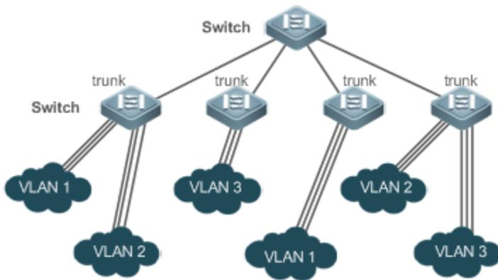
You may configure an Ethernet port or Aggregate Port (See *Configuring Aggregate Port* for details) as a Trunk port.
