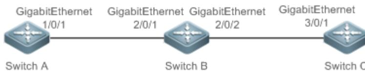
As shown in Figure 1-2, Switch A, Switch B, and Switch C form a simple L3 data communication network.
