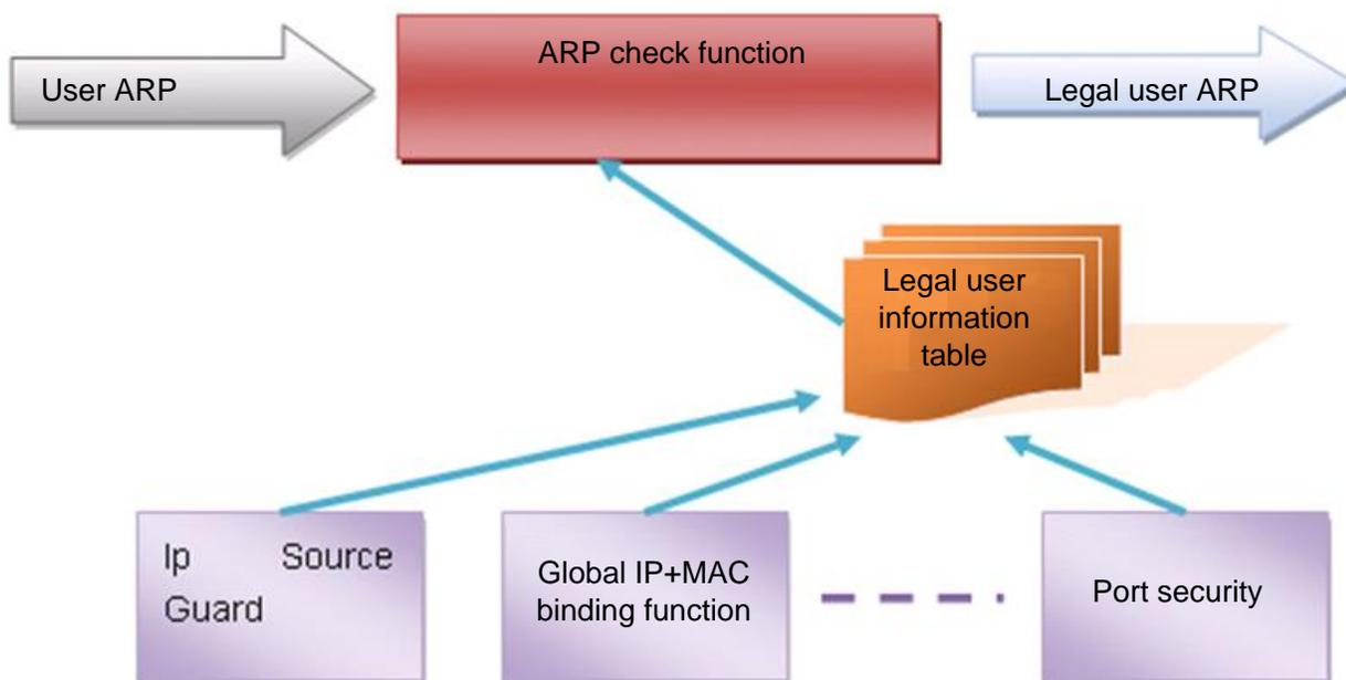
The above figure shows that security modules generate legal user information (IP-based or IP-MAC based). ARP Check uses the information to detect whether the Sender IP fields or the <Sender IP, Sender MAC>fields in all ARP packets at ports matches those in the list of legal user information. If not, all unlisted ARP packets will be discarded.
