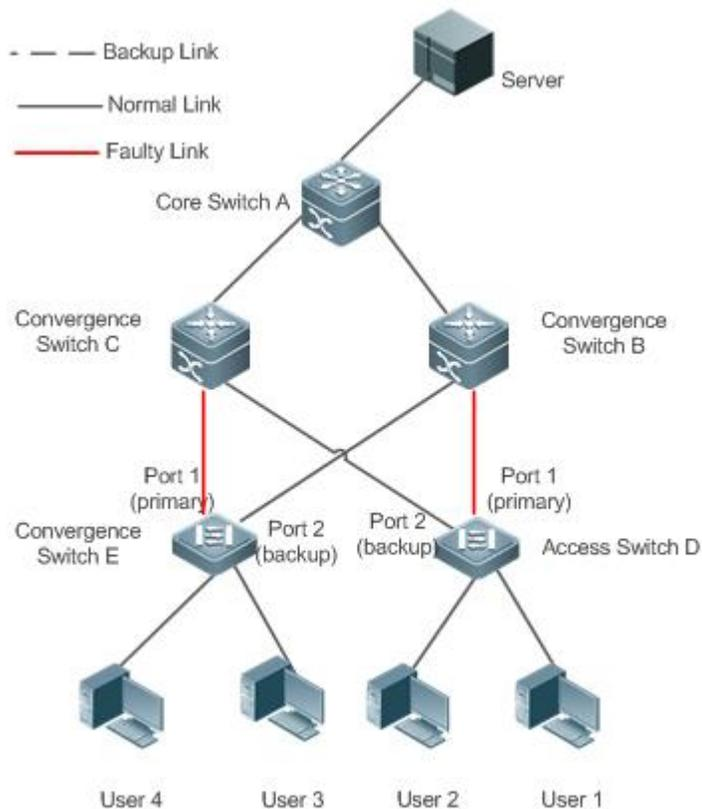
Once interface 1 is faulty, interface 2 immediately starts forwarding data packets and recovers the uplink transmission of the switch. In the non-preemption mode, when the link of interface 1 is recovered, interface 1 is in the backup state and does not forward data packets whereas interface 2 continues forwarding data packets.
