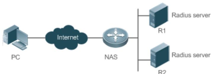
Figure 1-3 shows a typical AAA network topology, where two RADIUS servers (R1 and R2) and one NAS are deployed. The NAS can be the client for the RADIUS servers.
