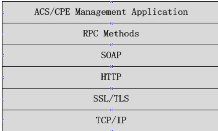
As shown in Figure 7-2, CWMP defines six layers with respective functions as follows:
