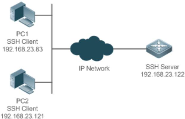
SSH users can use the local line password for user authentication, as shown in Figure 11-13. To ensure security of data exchange, PC 1 and PC 2 function as the SSH clients, and use the SSH protocol to log in to the network device where the SSH server is enabled. The requirements are as follows:
