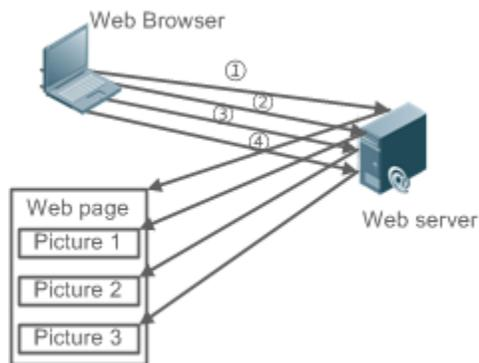
HTTP/1.1 overcomes the defect. It supports persistent connection, that is, one connection can be used to transmit multiple requests and response messages. In this way, a client can send a second request without waiting for completion of the previous request. This reduces network delay and improves performance. See the following figure:
