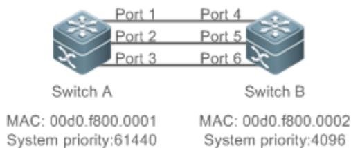
In Figure 3-2, Switch A is connected to Switch B through three ports. Set the system priorities of Switch A and Switch B to 61440 and 4096 respectively. Enable LACP on the Ports 1–6, set the aggregation mode to the active mode, and set the port priority to the default value 32768.
