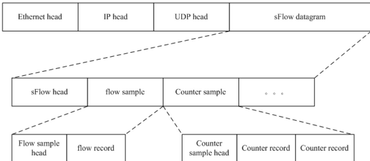
One sFlow datagram may contain one or multiple flow samples and counter samples.
