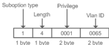
Relay agent information option82: This scheme serves without correlation with other protocol modules. A DHCP relay agent forms an Option 82 based on the physical port receiving DHCP request packets and the MAC address of the device. The option format is shown in the following figure.
