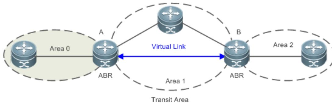
As shown in Figure 3-4, a virtual link is set up between A and B to extend Area 0 to B so that Area 0 can be directly connected to Area 2 on B. Area 1 is a transit area, A is an ABR of Area 1, and B is an ABR of Area 0 and Area 2.
