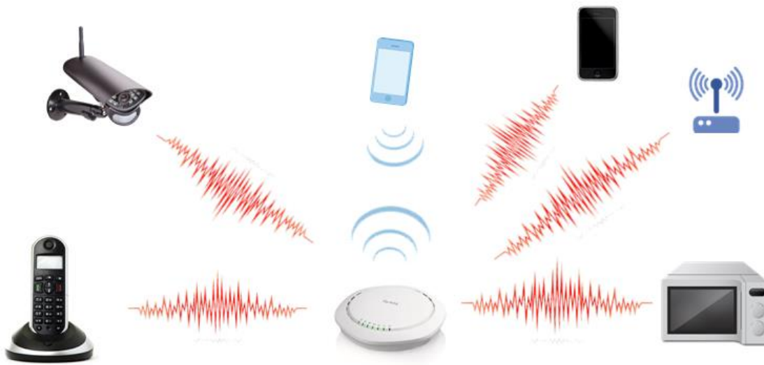
Figure 2. Interference result from non-Wi-Fi devices, other access points or nearby clients.
