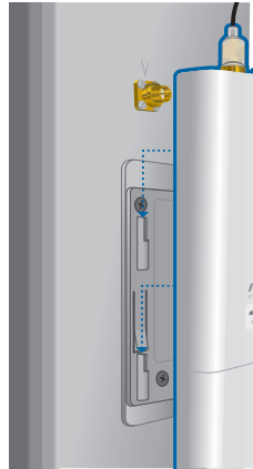
Mounting on a Sector Antenna
