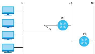
Figure 18 Example of Static Routing Topology
