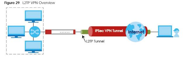
The Layer 2 Tunneling Protocol (L2TP) works at layer 2 (the data link layer) to tunnel network traffic between two peers over another network (like the Internet). In L2TP VPN, an IPSec VPN tunnel is established first (see Chapter 33 on page 278 for information on IPSec) and then an L2TP tunnel is built inside it.
