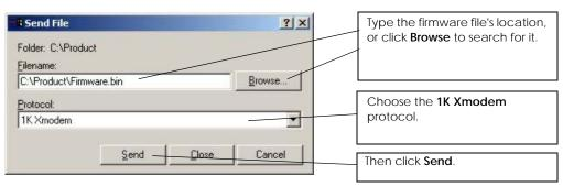
Figure 53 Example Xmodem Upload
