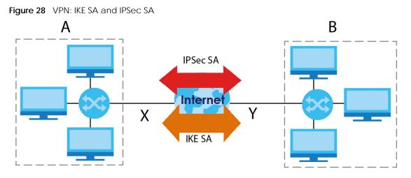
In this example, a computer in network **A** is exchanging data with a computer in network **B**. Inside networks **A** and **B**, the data is transmitted the same way data is normally transmitted in the networks. Between routers **X** and **Y**, the data is protected by tunneling, encryption, authentication, and other security features of the IPSec SA. The IPSec SA is secure because routers **X** and **Y** established the IKE SA first.
