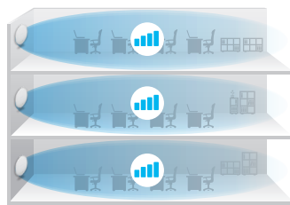
Dual-optimized (Side View) Pattern for wall-mount (H-plane, side view)
