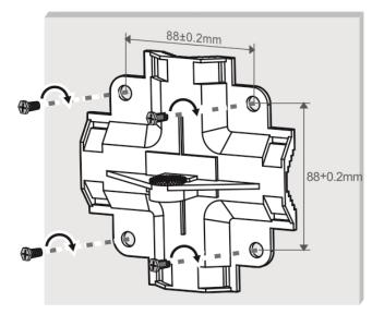
b. Hang the AP with the AP-side mounting bracket module to the cross-shaped bracket and tighten three M8×40 screws to secure the AP. Finally, drive the screw of Loop B into the fourth anchor. See Figure 3-5.
