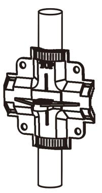
b. Attach the mounting plate to the mounting bracket through the rod with the M8x40 screws, adjust AP orientation, and tighten the screws on the rod with the Phillips screwdriver (or the wrench). Finally, connect Loop B of the security cable to the bracket by fastening the screw attached to Loop B. See Figure 3-7.
