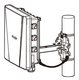
Figure 3-11 Clockwise Vertical Rotation (+60°)
