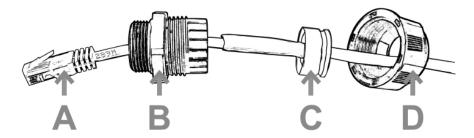
4) Insert the plug into the PoE IN port and tighten B, C and D in order.
