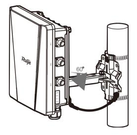
Figure 3-9 Clockwise Horizontal Rotation (+60°)
