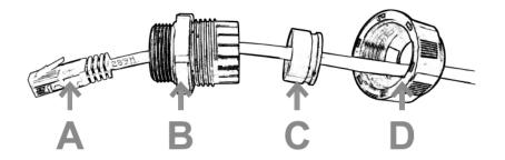
3) Wrap the cable between B and C upwards with two or three layers of liquid-tight material. See Figure 3-15.
