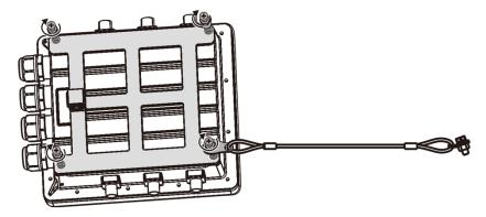
Attach the tie rod to the mounting plate and fasten the rod with the M8x40 screws after AP is well-positioned See Figure 3-3.
