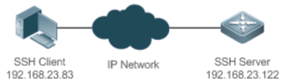
Figure 11-4 Network Topology for Public Key Authentication of SSH Users
