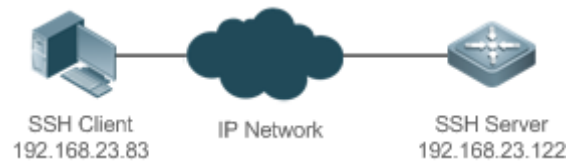
Figure 11-5 Networking Topology of SSH File Transfer
