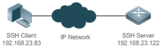
Figure 11-1 Networking Topology of SSH Device Management
