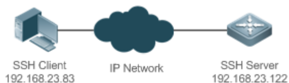
Figure 15-1 Networking Topology of SSH Device Management
