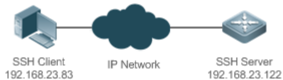
Figure 15-5 Networking Topology of SSH File Transfer
