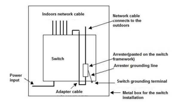
A The Ethernet port arrester is only for the 10M/100M copper Ethernet ports with the RJ45 connector;
