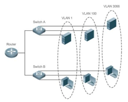
The VLANs supported by Ruijie products comply with the IEEE802.1Q standard. A maximum of 4094 VLANs (VLAN ID 1-4094) are supported, among which VLAN 1 cannot be deleted.
