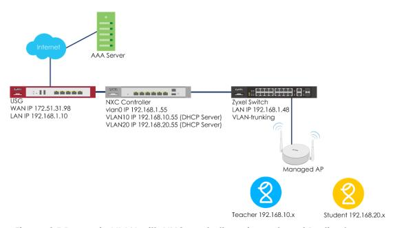
Figure 4.5 Dynamic VLAN with NXC controller using external Radius Server
