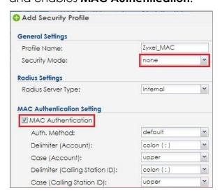
2 Go to CONFIGURATION > Object > AP Profile > SSID > SSID List, Create the SSID profile with the security profile.
