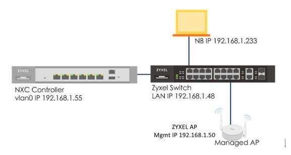
Figure 7.3 Upgrade AP firmware via GUI
