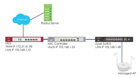
Figure 4.1 Set up AP/NXC with an External Radius Server
