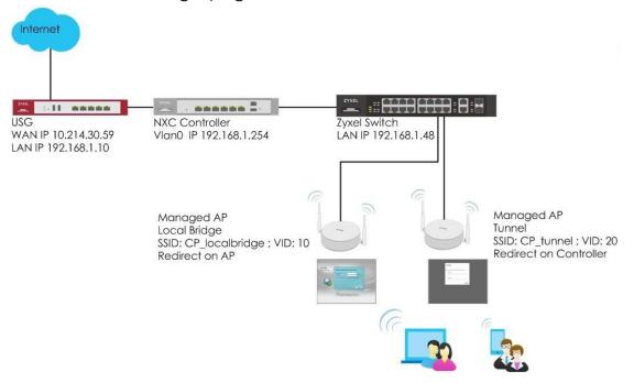
Figure 5.5 multiple captive portal for different users
