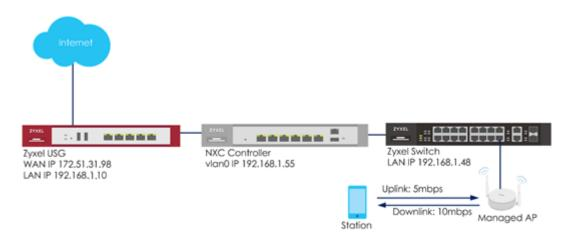
Figure 3.3 Uplink and Downlink Rate Limiting per Station
