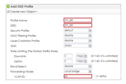
2 Go to CONFIGURATION > Object > AP Profile > SSID > Security List, Click Add to add the security profile for employees. Key in the Profile Name and SSID to employee. Click OK to save.
