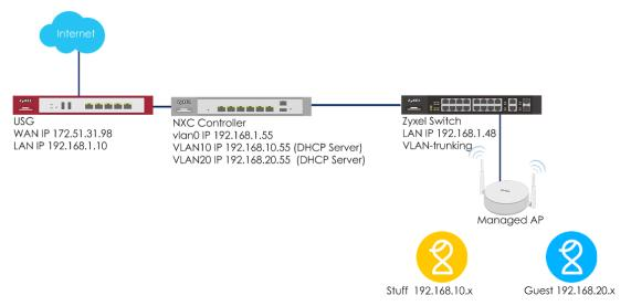
Figure 2.2.1 Set Different VLANs for Different SSIDs When USG is DHCP Server
