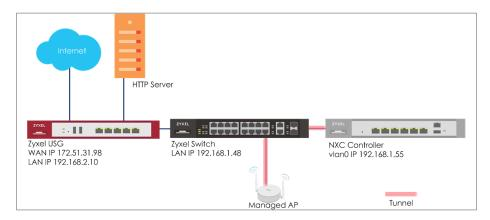
4 When using the NXC2500 as the controller, the uplink port MUST be ge1.
