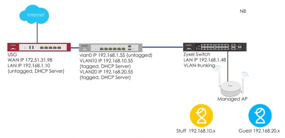
Figure 2.2.2 Set different VLANs for different SSIDs when NXC is DHCP server
