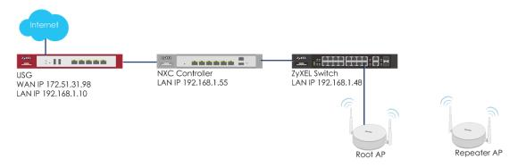
Figure 2.4 Setup ZyMesh for Root AP and Repeater AP
