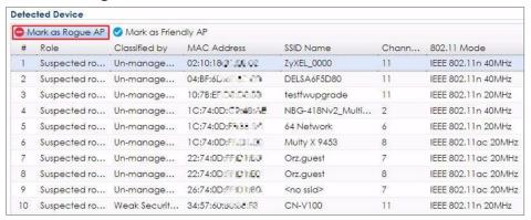
When the AP is marked as a rogue AP, it can be set in the containment list in CONFIGURATION > Wireless > Rogue AP > Rogue/Friendly AP List and the stations are difficult to connect with the containment AP.
