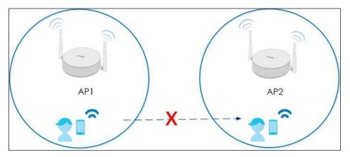
When AP1 and AP2 overlapping is too large, the AP1 and AP2's signal are interference to each other. Here are two ways for solving this issue. One is to make these two APs more far away from each other; the other is to decrease Max output power.
