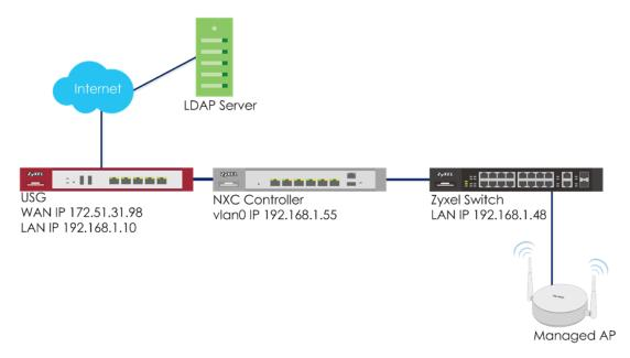
Figure 4.3 Set up AP/NXC with an External LDAP Server
