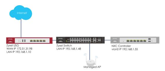
Figure 5.1.a Captive portal redirect on controller (USG is gateway)
