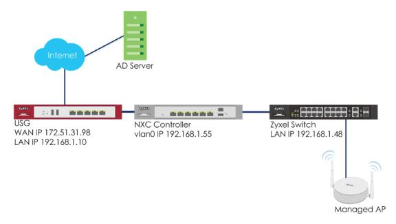
Figure 4.2 Set up AP/NXC with an External AD Server
