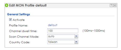
2 Configure AP to monitor mode in CONFIGURATION > Wireless > AP Management. Select the AP which is going to work in monitor mode and click Edit to change. Check Override Group Radio Setting and select MON Mode with default radio 1 profile which is set in step 1. Click OK to save.
