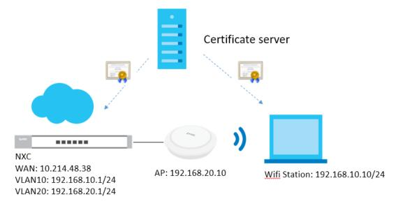
Figure 4.7 Use 802.1x with EAP-TLS
