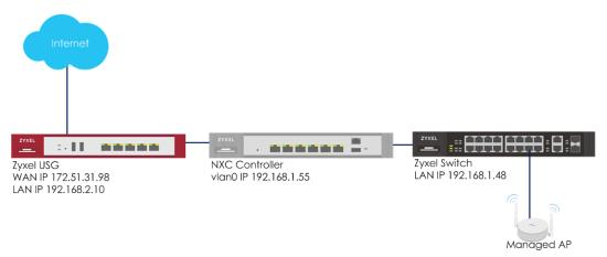
Figure 5.1.b Captive portal redirect on controller (NXC is gateway)
