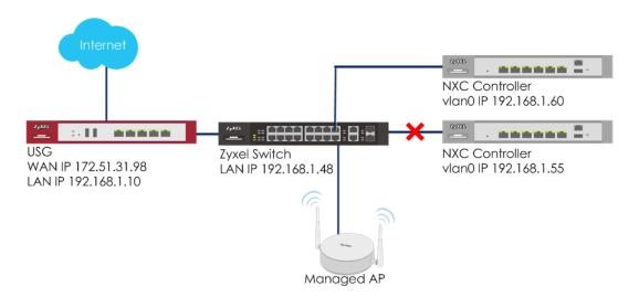
Figure 2.3 Fail Over and Fall Back
