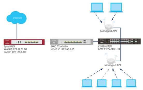
Figure 11 Load Balance
