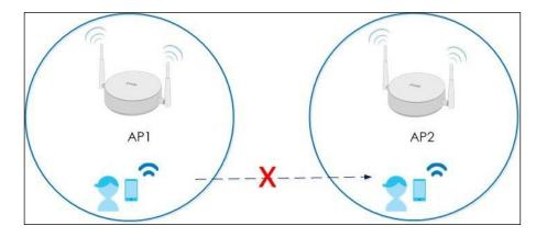
2 When AP1 and AP2 overlapping is too large, the AP1 and AP2's signal are interference to each other. Here are two ways for solving this issue. One is to make these two APs more far away from each other; the other is to decrease Max output power.
