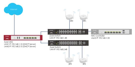
Figure 1.1 Manage APs through NXC Controller
