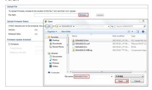
3 In MAINTENANCE > File Manager > Firmware Package, click Upload...to start to upload the firmware.
