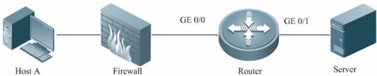
Figure 20 Networking topology for a terminal to access the server through the router and firewall
