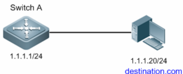
Figure1 Networking topology for static DNS configuration
