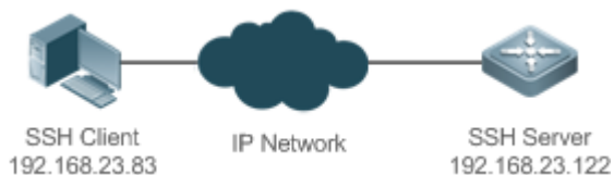
Figure 15-1 Networking Topology of SSH Device Management
