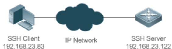
Figure 15-5 Networking Topology of SSH File Transfer
